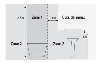
This product is suitable for use in Zone 2 and outside Zones of a bathroom. See diagram. If this unit is being fitted in Zone 1 a room containing a bath or shower, a 30mA RCD must be used, in accordance with IEE regulations.
